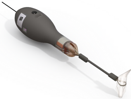
Figure 1— sPAT tag rigged with a stainless- steel heat shrink-covered tether and a Wilton anchor.
