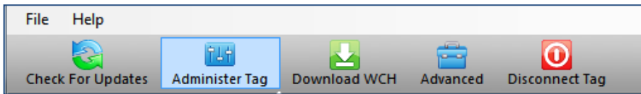
Figure 6—Tag Agent menu bar. Select Administer Tag to edit tag release settings.
