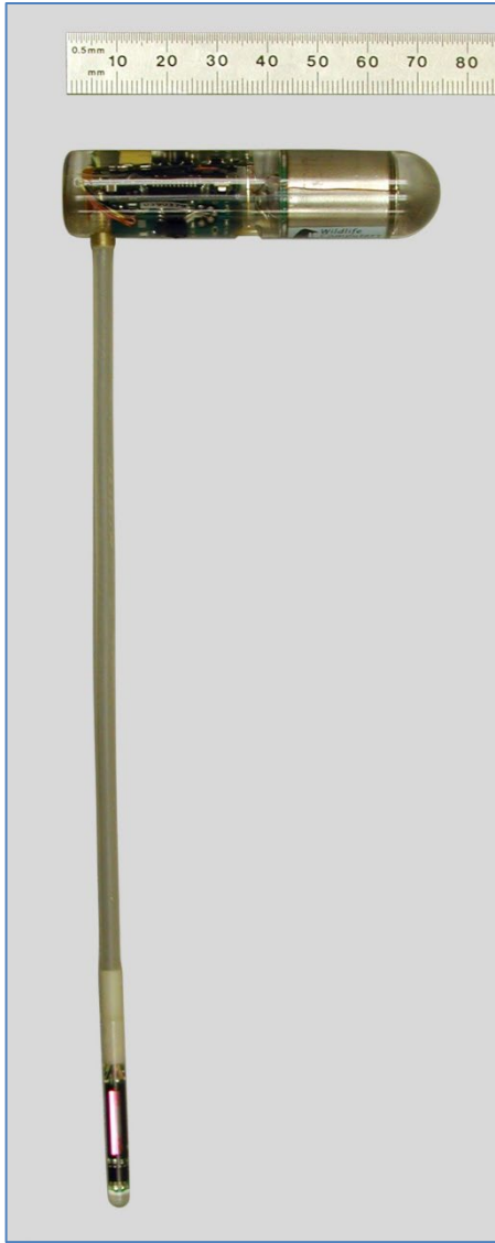
Left: Example of an implantable Mk9 tag in the L-configuration with light sensor and one of two temperature sensors in the stalk.
