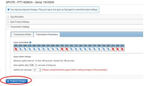
the tag is connected to Tag Agent through the USB communications cable, a pop-up box will alert you to load the newly selected settings into the tag.
