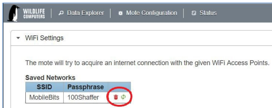
Figure 21—Removing and reconnecting a WiFi network
