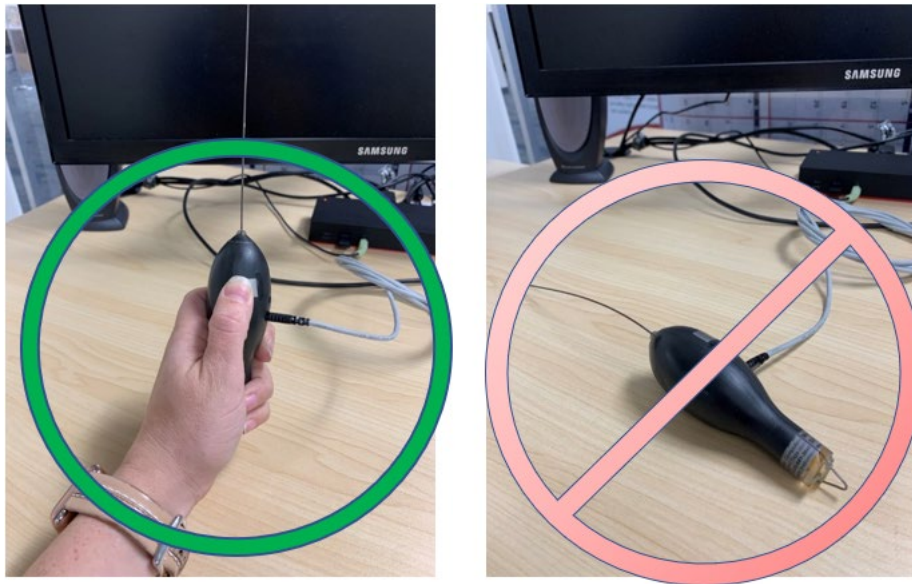
Figure 24—Optimal orientation of pop-up tag for Test Transmission.
