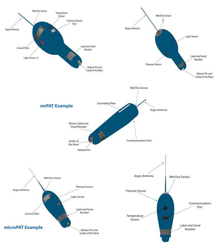
For Micron-painted tags, you will need to paint the following sensors with one coat of Propspeed:
